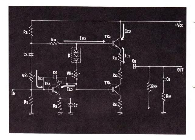
A BIAS VOLTAGE IS GIVEN TO TRANSISTOR 2 FROM THE CENTER POINT THROUGH VR<sub>1</sub> which is for regulating the center VOLTAGE. THEN THE COLLECTOR CURRENT FOR TRANSISTOR 2, OR  $I_{C2}$ , STARTS TO FLOW, AND THE COLLECTOR VOLTAGE, OR V<sub>C2</sub>, DROPS.
