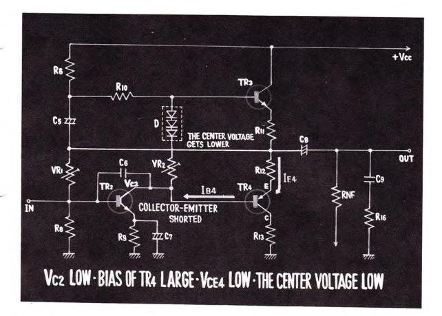
WHEN THE COLLECTOR AND THE EMITTER OF TRANSISTOR 2 ARE SHORTED, THE COLLECTOR VOLTAGE OF TRANSISTOR 2 BECOMES LOW, THUS THE BIAS VOLTAGE OF TRANSISTOR 4 BECOMES LARGER. THEN, THE VOLTAGE DROP BETWEEN THE COLLECTOR AND THE EMIT-TER OF TRANSISTOR 4 GETS SMALLER. THEREFORE, THE CENTER VOLTAGE ALSO GETS LOWER.
