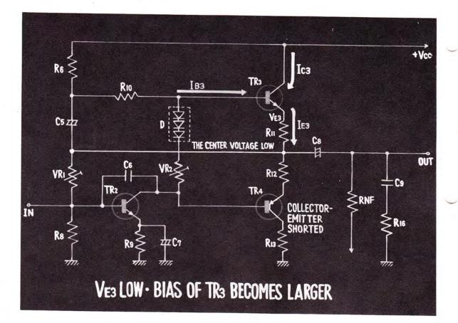
IT SHOULD BE EMPHASIZED THAT IN THIS CASE, AS THE COLLECTOR AND THE EMITTER OF TRANSISTOR 4 GET SHORTED THE TRANSISTOR 3 MAY ALSO BE DAMAGED DUE TO INCREASE IN BIAS OF TRANSISTOR 3.
