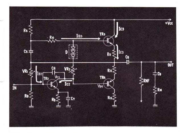
THE COLLECTOR OF TRANSISTOR 2 IS DIRECTLY CONNECTED TO THE BASE OF TRANSISTOR 4 SO THAT THE BASE VOLTAGE, OR  $V_{B4}$ , OF TRANSISTOR 4 ALSO DROPS.
