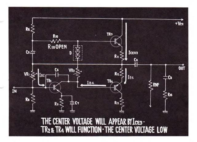
IN THIS CASE, IT MAY SEEM THAT NO VOLTAGE IS PRODUCED AT THE CENTER POINT SINCE NO BIAS VOLTAGE IS APPLIED TO TRANSISTOR 3. HOWEVER, ACTUALLY, A VOLTAGE IS PRODUCED AT THE CENTER POINT BECAUSE OF  $I_{CEO3}$ , THE COLLECTOR CUT-OFF CURRENT OF TRANSISTOR 3, WHICH IS THE COLLECTOR-EMITTER CURRENT WHEN THE BASE IS OPEN.
