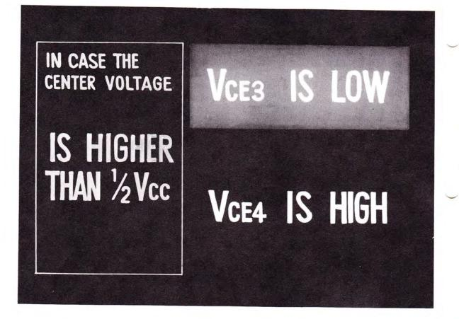
WHEN THE CENTER VOLTAGE IS HIGHER THAN 1/2  $V_{cc}$ , IT MAY BE THAT THE VOLTAGE BETWEEN THE COLLECTOR AND THE EMITTER OF TRANSISTOR 3, OR  $V_{ce3}$ , IS LOW, OR, ON THE CONTRARY, IT MAY BE THAT THE VOLTAGE BETWEEN THE COLLECTOR AND THE EMIT-TER OF TRANSISTOR 4, OR  $V_{ce4}$ , IS HIGH.
