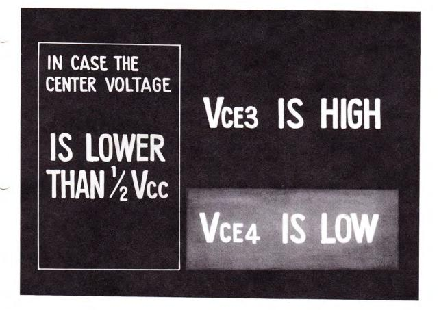
WHEN THE CENTER VOLTAGE IS LOWER THAN 1/2  $V_{cc}$ , IT MAY BE THAT THE VOLTAGE BETWEEN THE COLLECTOR AND THE EMITTER OF TRANSISTOR 3, OR  $V_{CE3}$ , IS HIGH, OR IT MAY BE THAT THE VOLT-AGE BETWEEN THE COLLECTOR AND THE EMITTER OF TRANSISTOR 4, OR  $V_{CE4}$ , IS LOW.
