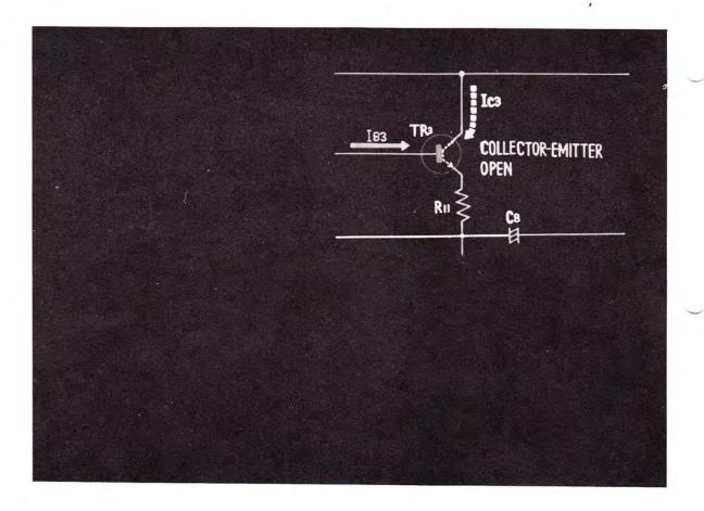
IT MAY SEEM THAT WHEN THE COLLECTOR AND THE EMITTER OF TRANSISTOR 3 IS OPEN, NO VOLTAGE WOULD APPEAR AT THE CENTER POINT, BECAUSE NO COLLECTOR CURRENT FLOWS TO TRANSISTOR 3 EVEN THOUGH THE BIAS IS GIVEN TO IT.
