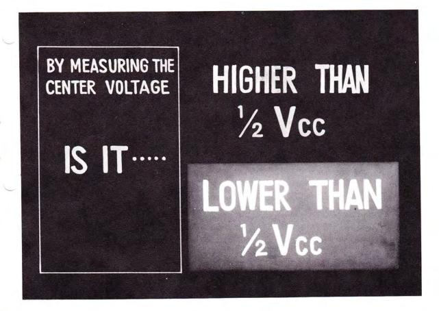
WHEN CHECKING THE COMPLEMENTARY MAIN AMPLIFIER CIRCUIT, FIRST, MEASURE THE CENTER VOLTAGE, AND THEN, CONSIDER SEPARATELY THE CASES WHERE IT IS HIGHER THAN THE NORMAL VALUE OF  $1/2 V_{cc}$  AND WHEN IT IS LOWER.
