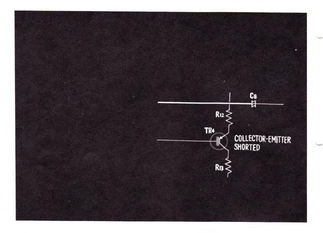
WHAT IF THE COLLECTOR AND THE EMITTER OF TRANSISTOR 4 ARE SHORTED?
