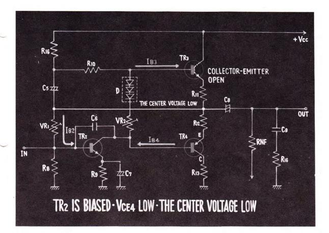
ACTUALLY, HOWEVER, VOLTAGE APPEARS AT THE CENTER POINT BY THE BASE CURRENT IN TRANSISTOR 3.
