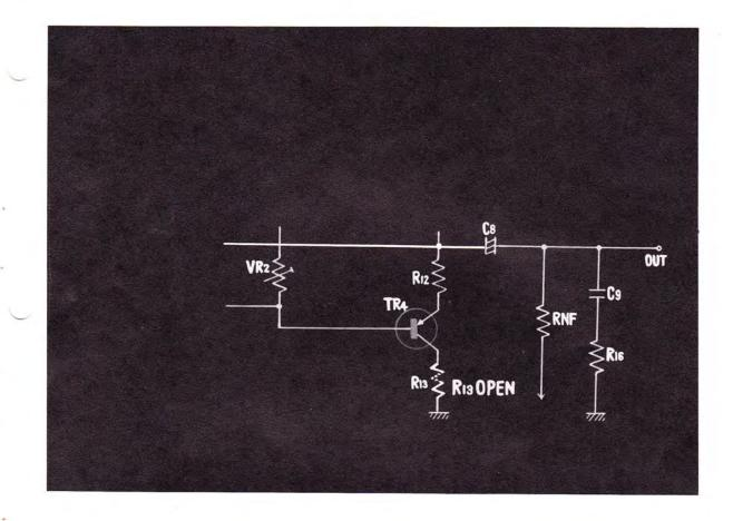
57. NEXT, WHAT ABOUT THE CASE WHEN THE RESISTOR  $R_{1\,3}$  IS OPEN?
