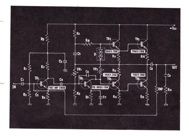
ON THIS BASIC DIAGRAM, TRANSISTOR 1 IS FOR THE PRIMARY-STAGE AMPLIFICATION, TRANSISTOR 2 IS FOR THE PRE-DRIVING PURPOSE, TRANSISTORS 3 AND 4 ARE FOR THE DRIVE-STAGE, AND TRANSISTORS 5 AND 6 ARE FOR THE POWER STAGE.
