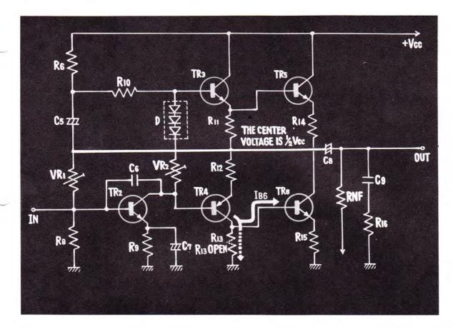
IF TRANSISTOR 6 IS CONNECTED IN THE CIRCUIT, THE COLLECTOR CURRENT OF TRANSISTOR 4 BECOMES THE BASE CURRENT OF TRANSISTOR 6, MAINTAINING THE CENTER VOLTAGE AT  $1/2 V_{CC}$ OR THE NORMAL VALUE.
