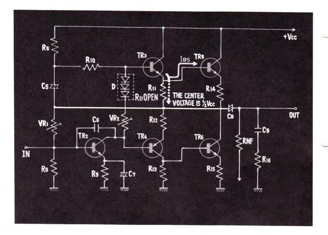
HOWEVER, IN ACTUAL CIRCUITS, TRANSISTOR 5 IS ALWAYS CONNECTED. THEREFORE, THE EMITTER VOLTAGE OF TRANSISTOR 3 BECOMES THE BASE CURRENT OF TRANSISTOR 5, MAINTAINING THE CENTER VOLTAGE AT  $1/2 V_{cc}$  OF THE NORMAL VALUE.
