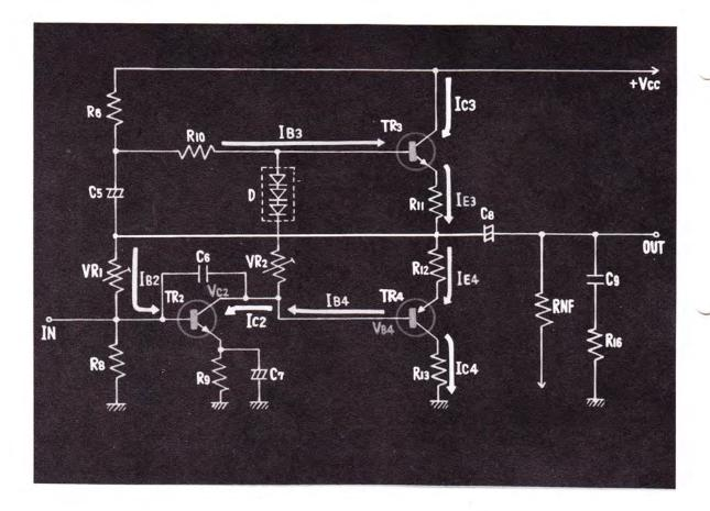
SINCE TRANSISTOR 4 IS A P-N-P TYPE, A BIAS VOLTAGE IS IN FACT GIVEN TO TRANSISTOR 4, AND CURRENT THUS FLOWS TO TRANSIS-TOR 4.
