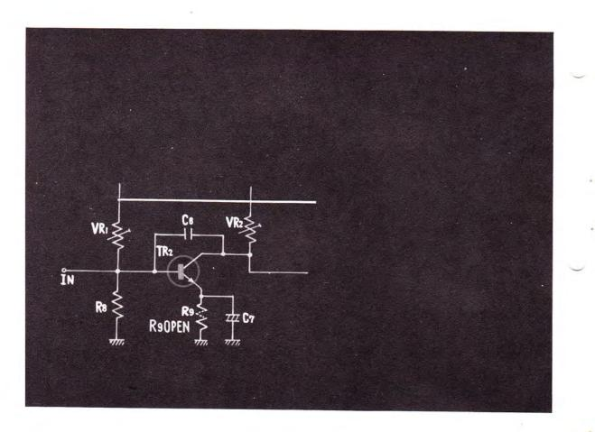
WHAT ABOUT THE CASE WHEN THE RESISTOR  $R_9\,$  IS OPEN?
