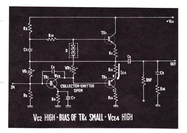
WHEN THE COLLECTOR AND THE EMITTER IS OPEN, THE COLLEC-TOR VOLTAGE OF TRANSISTOR 2 GETS HIGHER. AS A RESULT, THE BIAS FOR TRANSISTOR 4 BECOMES SMALL AND THE VOLTAGE BE-TWEEN THE COLLECTOR AND THE EMITTER RISES.
