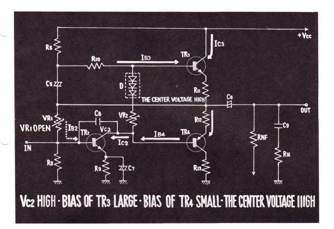
IF VR<sub>1</sub> IS OPEN, IT WILL NOT ALLOW TO GIVE BIAS VOLTAGE TO TRANSISTOR 2. THEREFORE, THE COLLECTOR CURRENT OF TRANSISTOR 2 DECREASES, CAUSING THE COLLECTOR VOLTAGE TO INCREASE.
