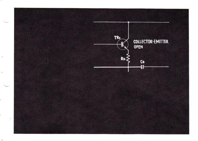
WHAT IF THE COLLECTOR AND THE EMITTER OF TRANSISTOR 3 IS OPEN?
