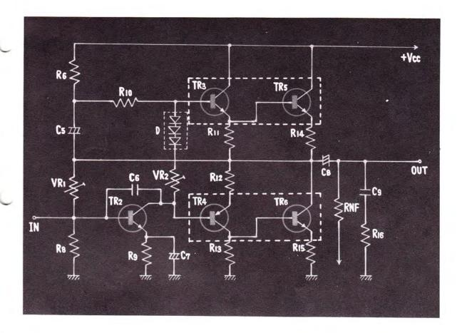
7. TRANSISTORS 3 AND 5 AS WELL AS TRANSISTORS 4 AND 6 ARE OF DARLINGTON-CONNECTION, SO THAT THEY MAY BE CONSIDERED AS N-P-N AND P-N-P TRANSISTORS, RESPECTIVELY.
