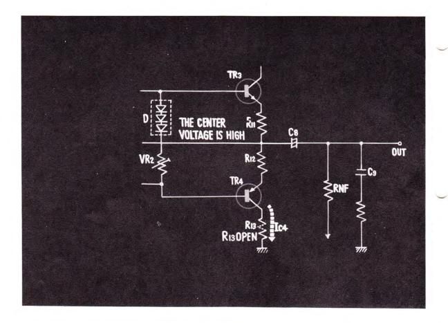
WHEN THE RESISTOR R<sub>13</sub> IS OPEN AND ALSO IF TRANSISTOR 6 IS NOT CONNECTED, THEN THE COLLECTOR CURRENT OF TRANSISTOR 4 BECOMES ZERO. AS A RESULT, THE CENTER VOLTAGE WILL GET HIGHER.
