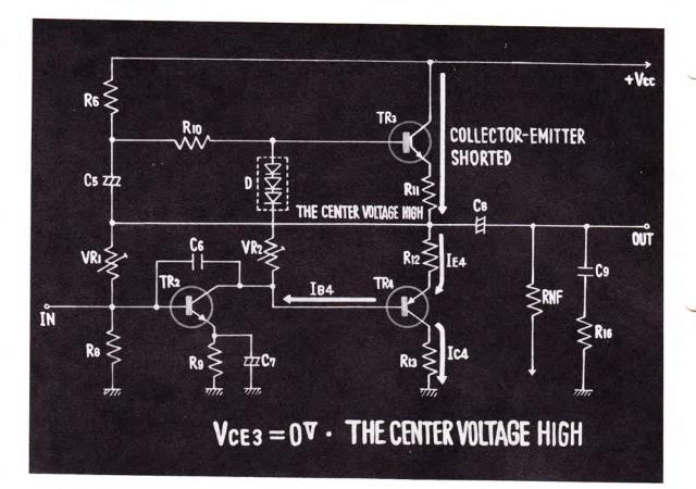
WHEN THE COLLECTOR AND THE EMITTER OF TRANSISTOR 3 BE-COME SHORTED, THE VOLTAGE BETWEEN THE COLLECTOR AND THE EMITTER BECOMES ZERO (OV), AND AS CURRENT FLOWS DIRECT-LY TO THE CENTER POINT FROM  $V_{cc}$  THROUGH R<sub>11</sub>, THE VOLTAGE AT THE CENTER POINT BECOMES HIGHER. IN THIS CASE, THE BIAS FOR TRANSISTOR 4 BECOMES LARGER, CAUSING AN INCREASE IN THE COLLECTOR CURRENT, THEREFORE, EVERY CAUTION IS NECESSARY TO PREVENT TRANSISTOR 4 FROM BEING DAMAGED.
