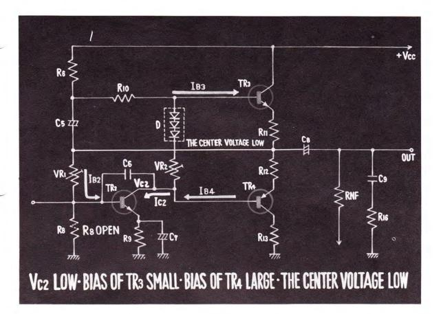
WHEN THE RESISTOR  $R_8$  IS OPEN, THE BIAS VOLTAGE OF TRANSISTOR 2 BECOMES LARGER, LOWERING THE COLLECTOR VOLTAGE. AC-CORDINGLY, THE BIAS VOLTAGE OF TRANSISTOR 3 BECOMES SMAL-LER, AND THAT OF TRANSISTOR 4 BECOMES LARGER, AND AS A RESULT, THE CENTER VOLTAGE BECOMES LOWER THAN 1/2 V<sub>cc</sub>.
