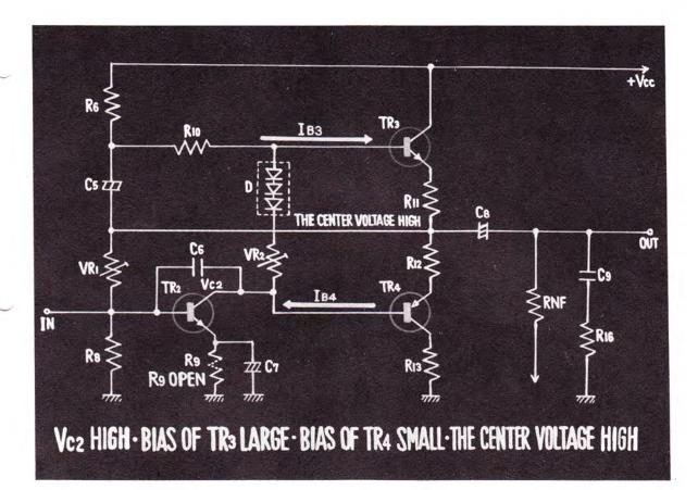
IN THIS CASE, NO CURRENT FLOWS INTO TRANSISTOR 2, MAKING ITS COLLECTOR VOLTAGE HIGHER. THE BIAS VOLTAGE OF TRANSISTOR 3 BECOMES LARGER, WHILE THAT OF TRANSISTOR 4 BECOMES SMALLER, AND AS A RESULT THE CENTER VOLTAGE BECOMES HIGHER THAN  $1/2 V_{cc}$ .
