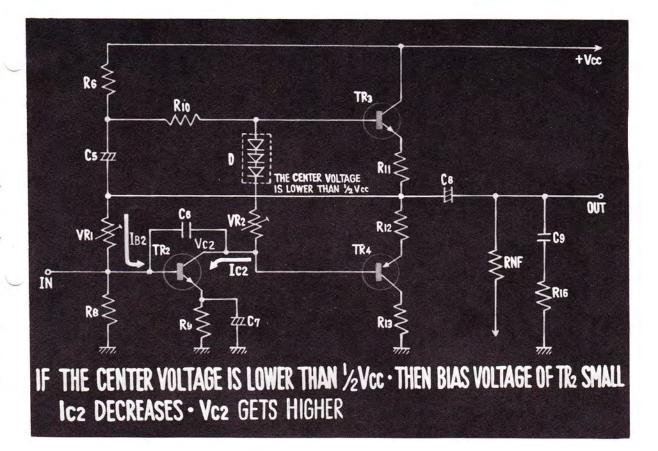
NOW, LET'S CONSIDER THE CASE WHERE THE CENTER VOLTAGE HAS DECREASED AND HAS BECOME LOWER THAN 1/2  $V_{cc}$ . THE BIAS VOLTAGE FOR TRANSISTOR 2 BECOMES INSUFFICIENT, BECAUSE OF THE DIRECT-CURRENT FEEDBACK FROM THE CENTER POINT THROUGH VR<sub>1</sub> TO TRANSISTOR 2. THE COLLECTOR CURRENT,  $I_{c2}$ , DECREASES AND THE COLLECTOR VOLTAGE  $V_{c2}$  GETS HIGHER.
