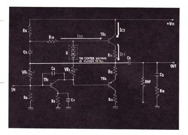
THE INSTANT V<sub>CC</sub> IS APPLIED, THE VOLTAGE AT THE CENTER POINT BECOMES ALMOST AS HIGH AS V<sub>CC</sub> ITSELF, BECAUSE A BIAS VOLTAGE IS GIVEN TO TRANSISTOR 3.
