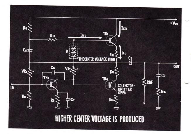
IN THIS CASE, NO CURRENT FLOWS BETWEEN THE COLLECTOR AND EMITTER, AND SINCE THE BIAS VOLTAGE IS APPLIED TO TRANSISTOR 3, A HIGH VOLTAGE APPEARS AT THE CENTER POINT.
