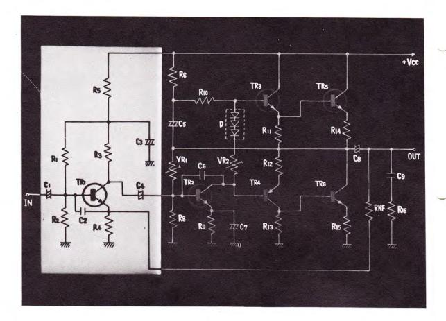
6. HERE, WE WILL OMIT FROM OUR STUDIES THE PRIMARY-STAGE AMPLIFIER SECTION OF TRANSISTOR 1, SINCE IT IS A VERY COMMON CIRCUIT OF CAPACITOR-COUPLED, EMITTER-GROUNDED TYPE.
