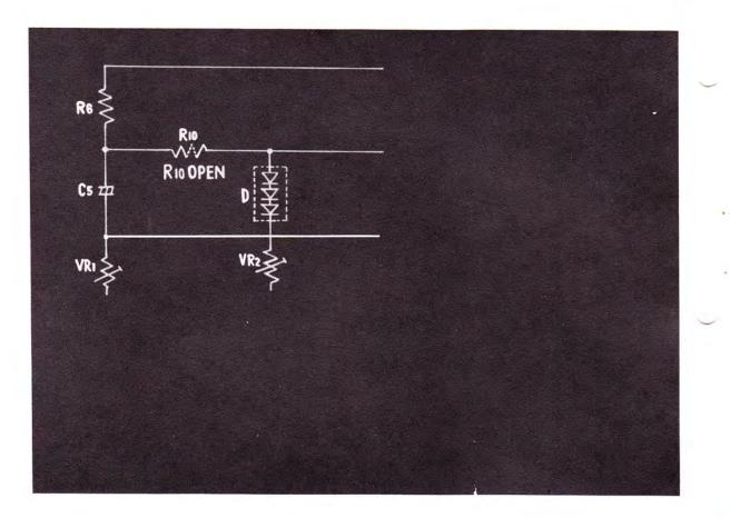
WHAT WILL HAPPEN WHEN THE LOAD RESISTOR R<sub>10</sub>OF TRANSISTOR 2 IS OPEN?
