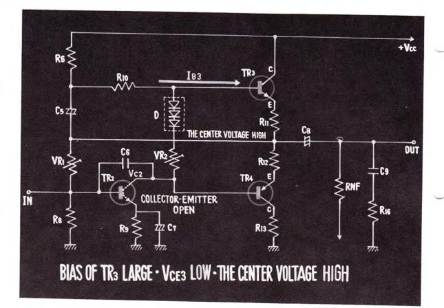
ON THE OTHER HAND, THE BIAS IN TRANSISTOR 3 BECOMES LARGER, AND THE VOLTAGE BETWEEN THE COLLECTOR AND THE EMITTER DROPS. AND THE CENTER VOLTAGE BECOMES HIGHER THAN THE NORMAL VALUE OF  $1/2 V_{cc}$ .
