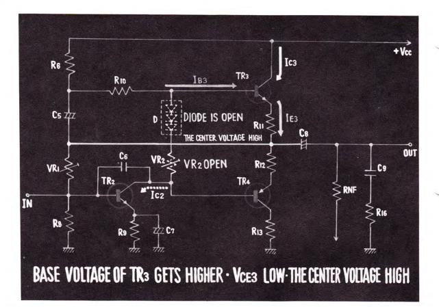
IN THIS CASE, THE COLLECTOR CURRENT OF TRANSISTOR 2 DOES NOT FLOW. THEREFORE, AS THE BASE VOLTAGE OF TRANSISTOR 3 INCREASES, THE BIAS VOLTAGE OF TRANSISTOR 3 GETS LARGER. CONSEQUENTLY THE VOLTAGE BETWEEN THE COLLECTOR AND EMIT-TER BECOMES LOWER, AND THE VOLTAGE AT THE CENTER POINT BECOMES HIGHER THAN  $1/2 V_{cc}$ .
