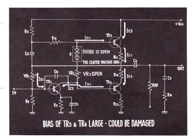
HOWEVER, SINCE THE BIAS VOLTAGE IS APPLIED TO TRANSISTOR 2, THE BASE CURRENT OF TRANSISTOR 4 FLOWS INTO THE COLLECTOR OF TRANSISTOR 2, MAKING THE BIAS VOLTAGE OF TRANSISTOR 4 LARGER. IN THIS CASE, EVERY CAUTION IS NECESSARY, BECAUSE A LARGE CURRENT FLOWS INTO TRANSISTORS 3 AND 4, CAUSING THEM TO BREAK DOWN.
