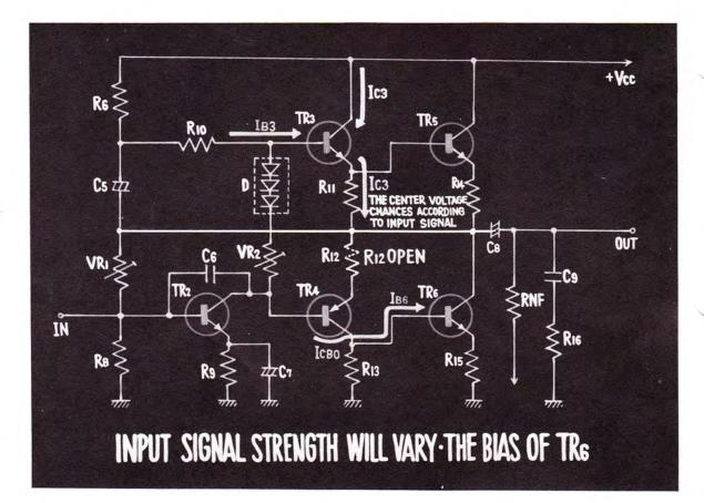
THIS  $I_{CEBO}$  OF TRANSISTOR 4 CHANGES DEPENDING UPON THE INPUT SIGNAL. ACCORDINGLY, THE BIAS VOLTAGE OF TRANSISTOR 6 ALSO CHANGES, THE CENTER VOLTAGE VARYING FROM HIGH TO NEAR 1/2 V<sub>CC</sub> IN ACCORDANCE WITH THE INPUT SIGNAL STRENGTH.
