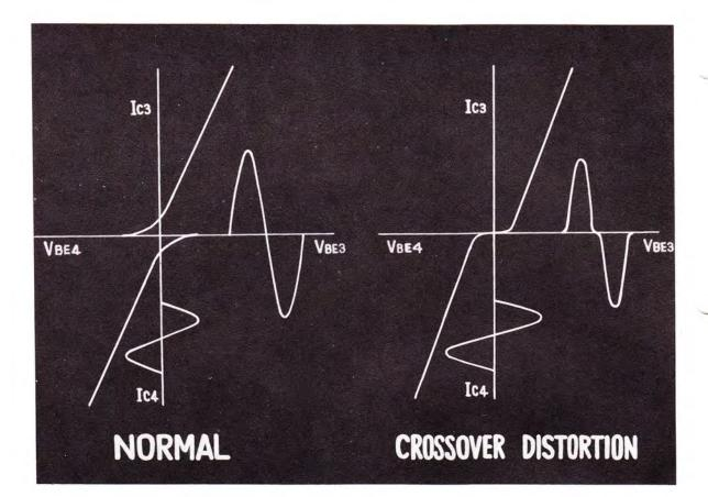
$^{38.}$  when the diode is shorted, the bias voltage in the drive-stage and power-stage becomes small, causing the function point shift onto the non-linear portion of the  $v_{\rm B} \cdot i_{\rm C}$  characteristic.
