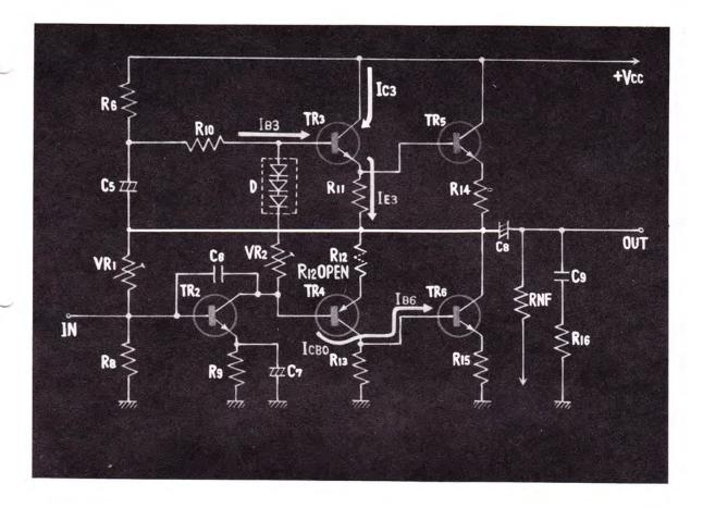
IF TRANSISTOR 6 IS CONNECTED IN THIS CIRCUIT, THE COLLECTOR BASE CURRENT  $I_{CEBO}$  WHEN THE EMITTER OF TRANSISTOR 4 IS OPEN BECOMES THE BASE CURRENT OF TRANSISTOR 6. HOWEVER, THIS VALUE OF  $I_{CEBO}$  IS EXTREMELY SMALL, THERE-FORE, THIS SERVES AS ALMOST NO BIAS FOR TRANSISTOR 6.
