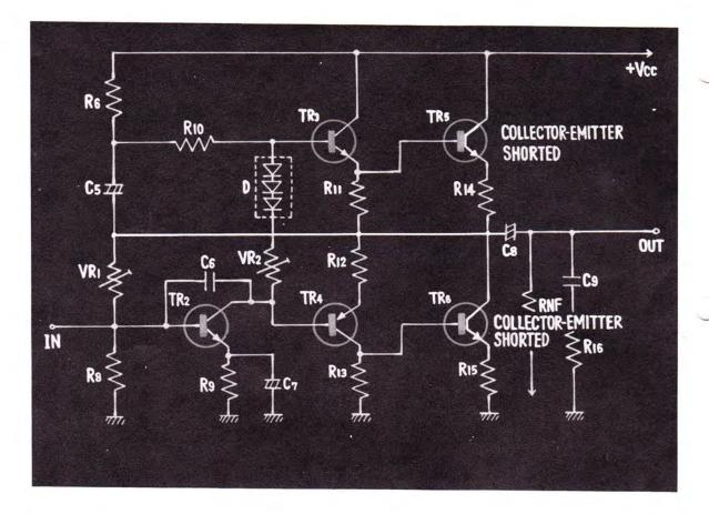
HOW ABOUT THE CASE WHEN POWER TRANSISTOR 5 OR 6 IS SHORT-ED? WHEN EITHER ONE OF THE POWER TRANSISTORS IS SHORTED, THE FUSE WILL BLOW IMMEDIATELY, MAKING IT IMPOSSIBLE TO CHECK THE CONDITION BY MEANS OF VOLTAGE.
